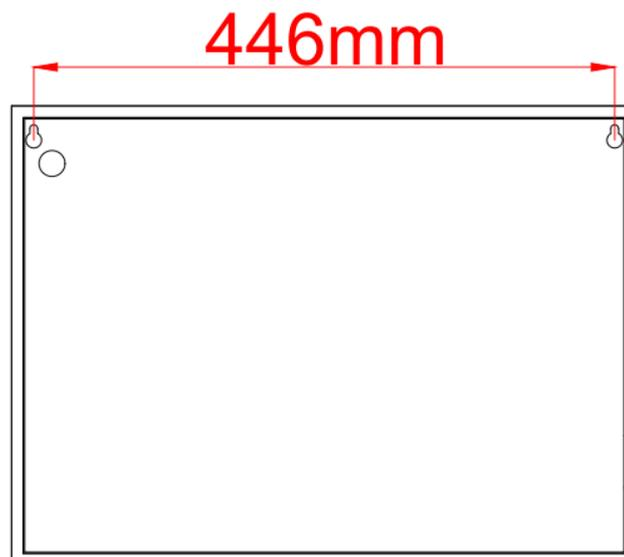
Mounting distance 446mm , Expansion bolt M5\*50\*2.
