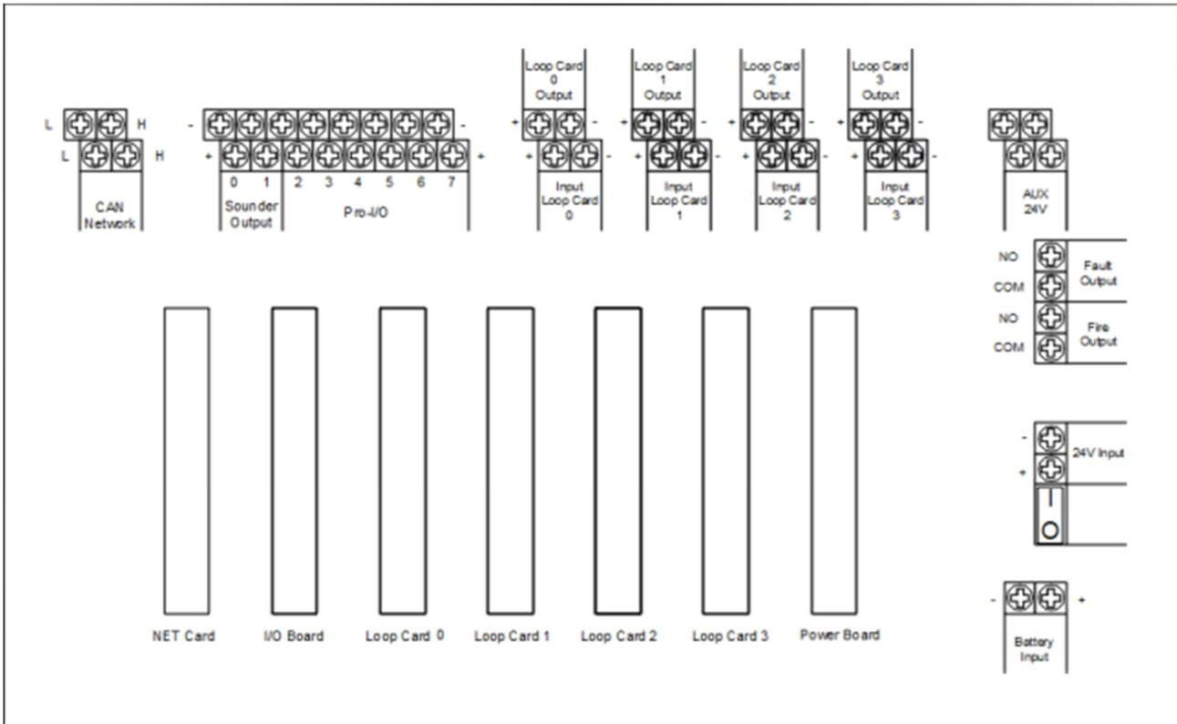
Fig. Terminal Board
