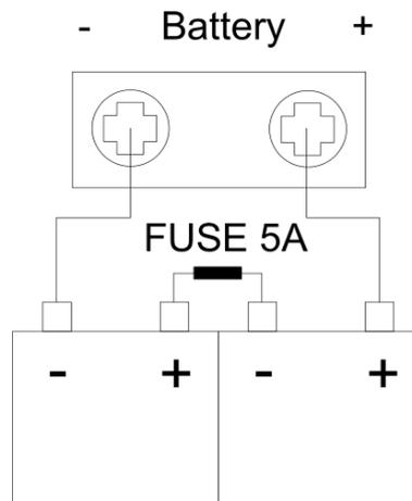
Fig. Battery Connection
