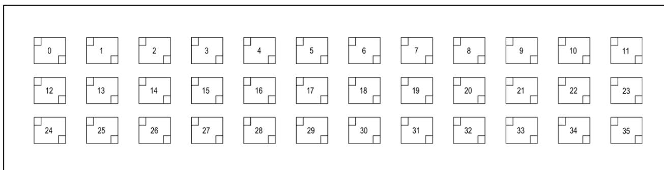
VI-6847 comes with 36 zone in one zone indication panel. On the indication panel, each unit consists of two indicators. User can put the name of device on the right side of the control panel.
