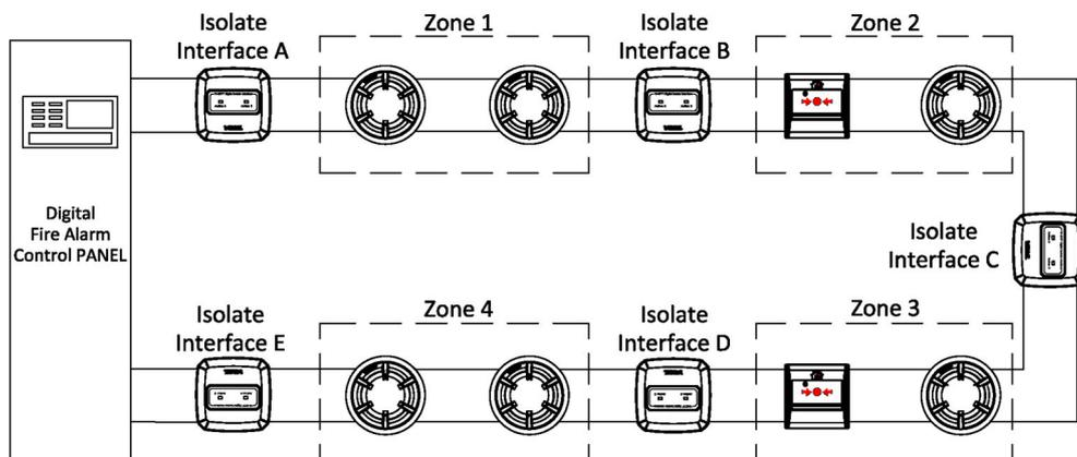
Fig. Loop device connection
