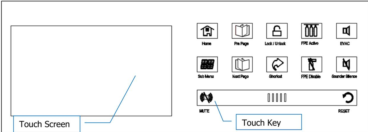
When do operation and setting on the touch screen, Touch keys are used for shortcut operations, here is touch key description in following table.
