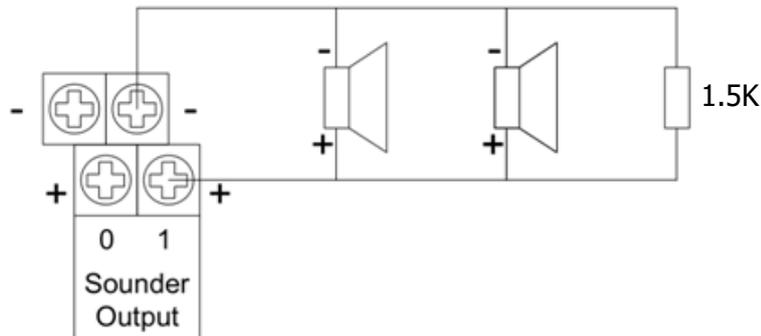
Fig.4-4. Connection of Sounder Output
